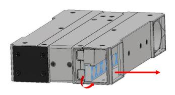
Before taking any access panel off, ensure the disconnect is turned to the "OFF" position. If the optional rotary bypass damper is installed, the filter can be removed by manually rotating the damper in the position shown below and sliding the filter out as indicated earlier. Note the damper rotates in only one direction.
