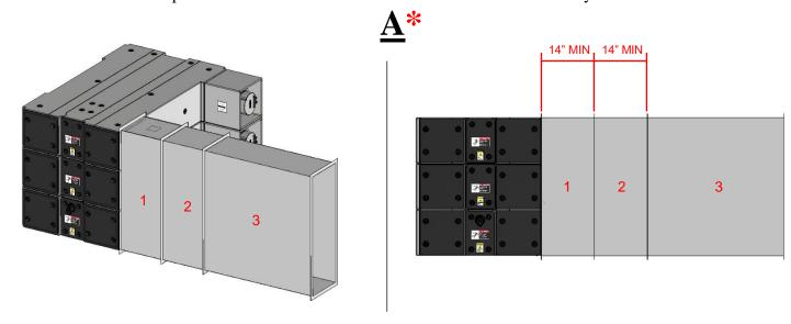
\*TO SERVICE A FAN WITHIN DUCT, REMOVE DUCT "2", FOLLOWED BY DUCT "1". ENSURE DUCT "3" IS INDEPENDENTLY SUPPORTED AND DOES NOT RELY ON THE SYSTEM FOR SUPPORT.
