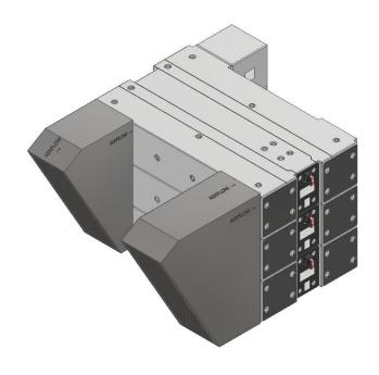
Once the intake is in place, secure it to the system flanges using #14 x 1.25" long self-drilling screws on all 4 sides. A minimum of 2 screws must be used per unit (i.e. an 1800 system requires at least 6 screws per intake)
