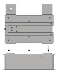
Place the remaining units (if applicable). Fasten the 4 connecting bolts inside each access panel with the hardware provided as shown
