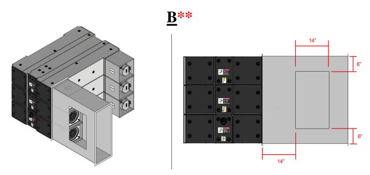
\*\*A WATER-TIGHT ACCESS PANEL CAN BE INSTALLED IN THE LOCATION AND SIZE SPECIFIED WITHIN THE DUCT TO SERVICE A FAN.
