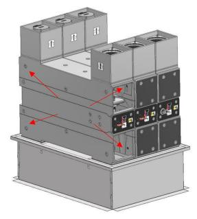
Once the system is in place, secure it to the curb duct flanges using #14 x 1.5" long self-drilling screws. A minimum of 4 screws must be used per unit (i.e. an 1800 system requires at least 12 screws)
