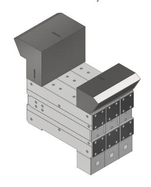
Once the intake is in place, secure it to the system flanges using #14 x 1.25" long self-drilling screws on all 4 sides. A minimum of 2 screws must be used per unit (i.e. an 1800 system requires at least 6 screws per intake)
