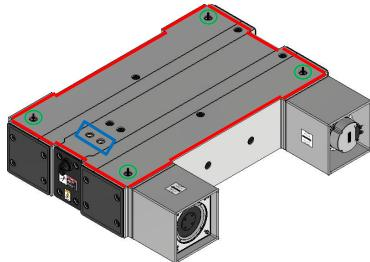
Prior to stacking the secondary unit with the primary, ensure the secondary unit electrical cabinet wire plugs are removed (blue) and receiving plugs w/ a 7/16" dia. hole are installed in each quadrant (green).
