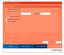
If the controller does not ask to install the upgrade file, access the controller system menu by holding the Alarm and Enter buttons for two seconds, then select the UPGRADE option. The software file should be listed. Once uploaded, power cycle the system.
