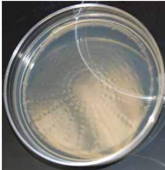
Figure 23: A typical plate immediately after removal from the viable samplers. The indents are caused by the air pressure forcing the microbes into the holes of the sampler stages.
