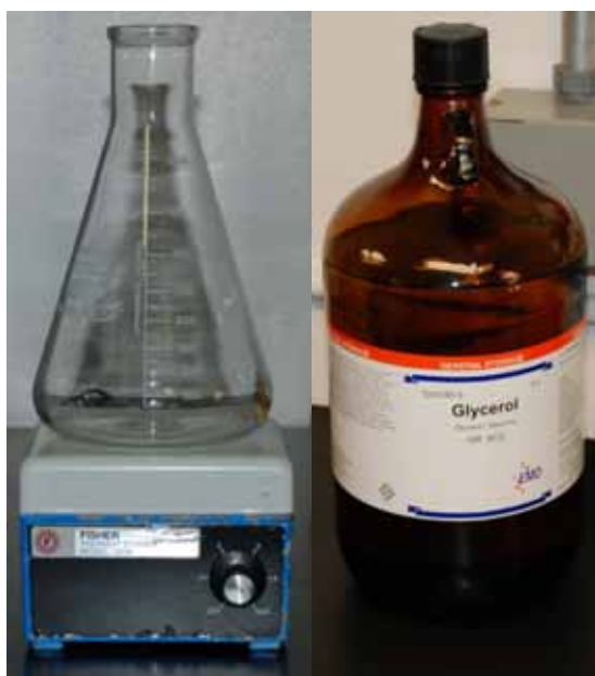
Figure B-2: a. Stirrer for use with boiling DG solutions; b. glycerol added to boiling solution.
