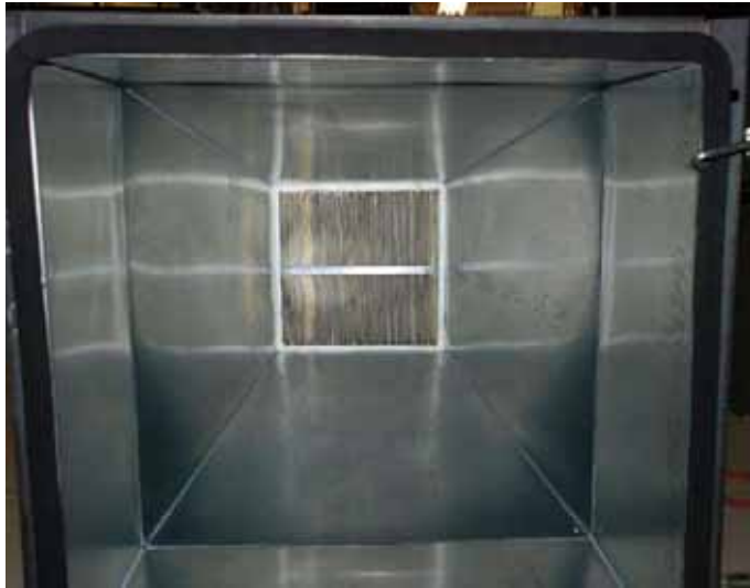
Figure 18: a. 52.2-compliant rig insert section used to house the Energy Wall core under test; b. Energy Wall fitted in the middle of the insert section using GE Silicone II XST sealant along the core perimeter to eliminate bypass around the perimeter of the core; c. inside view of insert without Energy Wall core installed.
