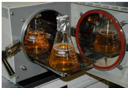
Figure A-5: Autoclave the prepared solutions in the 1000 ml flasks.
