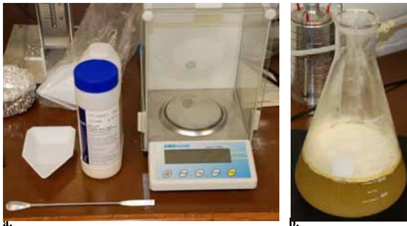
Figure A-2: a. Electronic scale and weighing equipment used to weigh agar powder; b. 2000 ml flask with the tryptic soy Agar.
