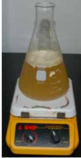
Figure A-3: Heating and stirring the agar solution on the magnetic stirrer/hot plate.
