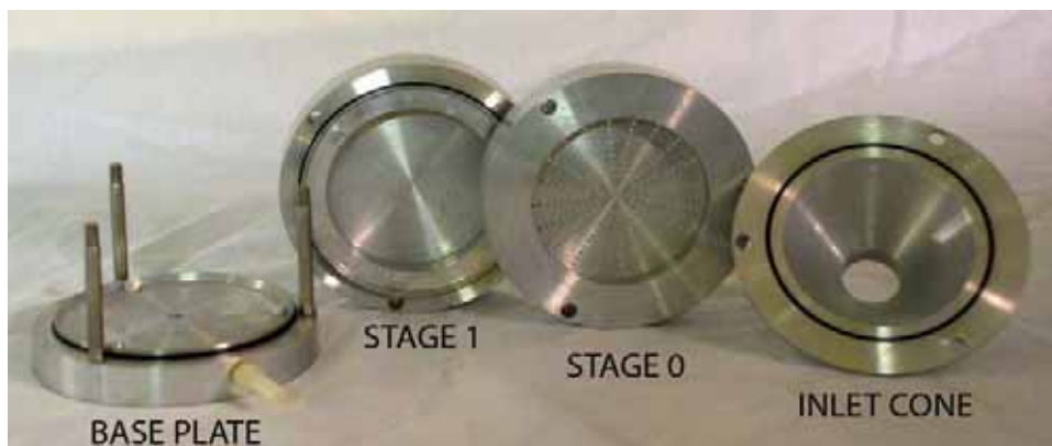
Figure 21: Two stage Anderson sampler assembly (pump and sampling lines not shown).
