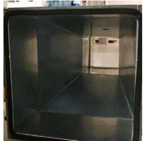
Figure 18: a. 52.2-compliant rig insert section used to house the Energy Wall core under test; b. Energy Wall fitted in the middle of the insert section using GE Silicone II XST sealant along the core perimeter to eliminate bypass around the perimeter of the core; c. inside view of insert without Energy Wall core installed.
