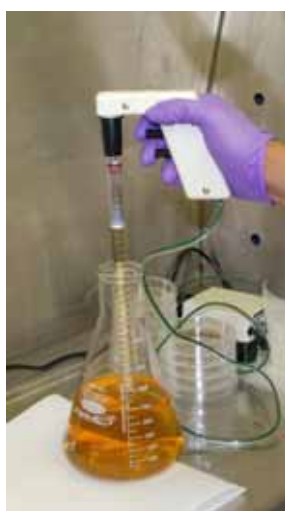
Figure C-3: Pipet-Aid device in use.
